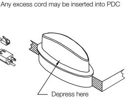
Slide the PDC onto work surface.
