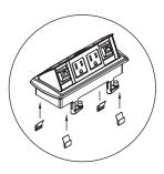
Use phillips head screwdriver to tighten locking cams snuglyto the work surface. To Access back screw, flip back power encloser past stops. After locking cam is secured, rotate power enclosure back into place. **Do not overtighten.**
