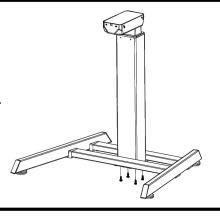
Using the supplied Allen Wrench, insert four (4) M6x14 Machine Screws (P11) through the holes in the Top Mounting Frame (P6) going into the top of the Leg (P1) and rotate each screw just a few turns.
